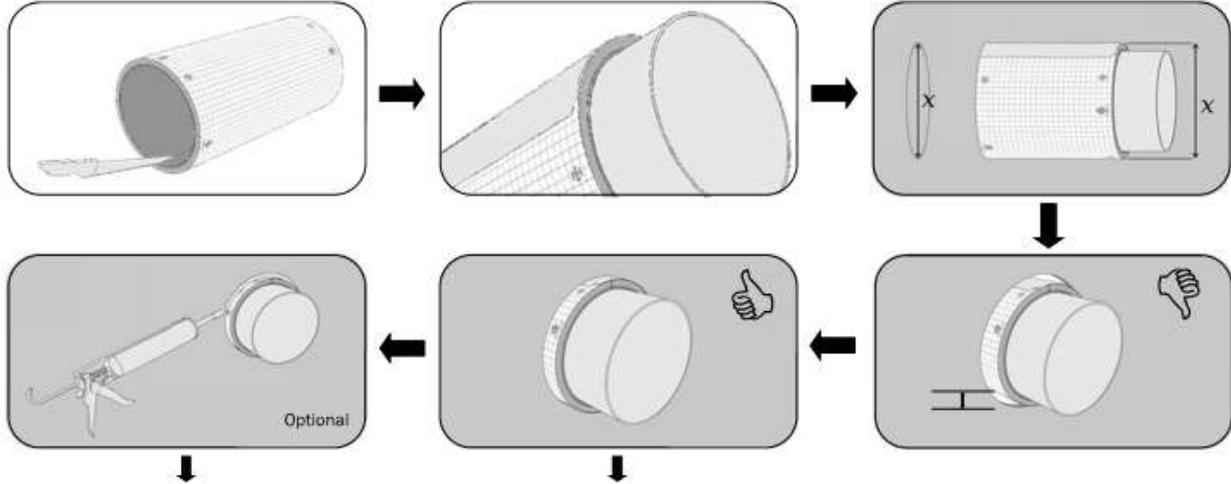
**Wall Penetrations - Plastic Vent Pipe / Ducting - Drywall Partition**
