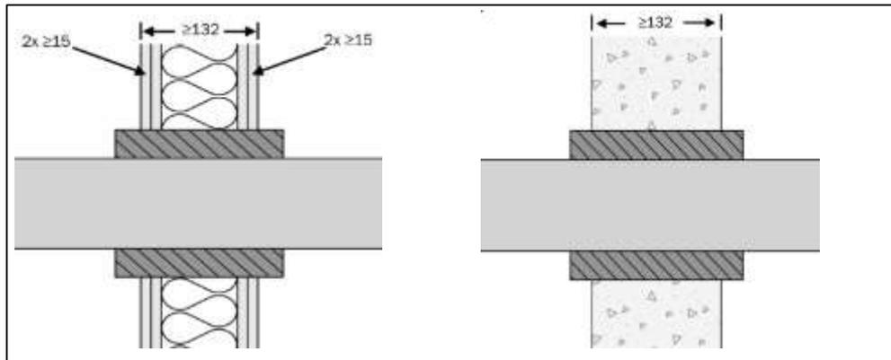
The seal must be a minimum of 180mm long with 24mm protruding each side of the wall
