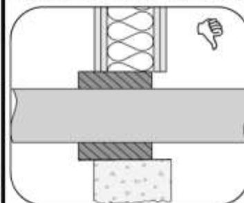
Rigid walls must comprise concrete, aerated concrete or masonry  $\ge 650$ kg/m<sup>3</sup> (Wall Type A) or concrete, masonry  $\ge 1100$ kg/m<sup>3</sup> (Wall Type B)
