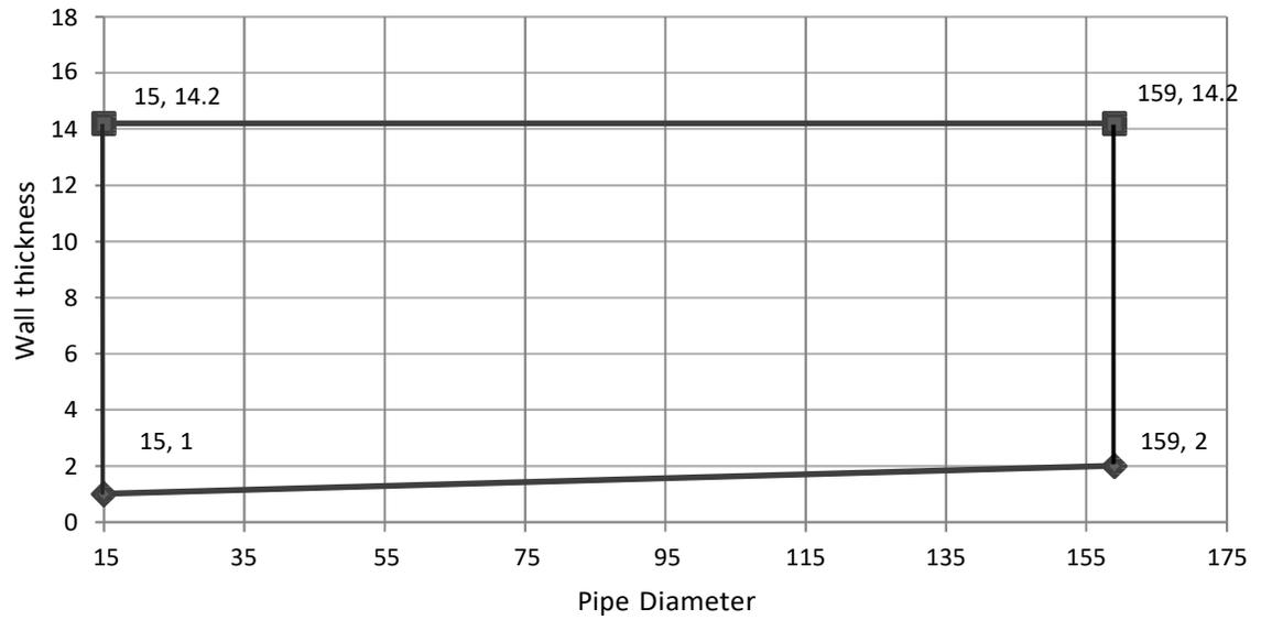
**B.2 Field of application for Tenmat Firefly 109 Fire Sleeve – Circular for PVC-U (according to EN 1329-1)\* and HDPE (according to EN 1519-1)\* pipes penetrating fire resistant walls for applications up to EI120:**
