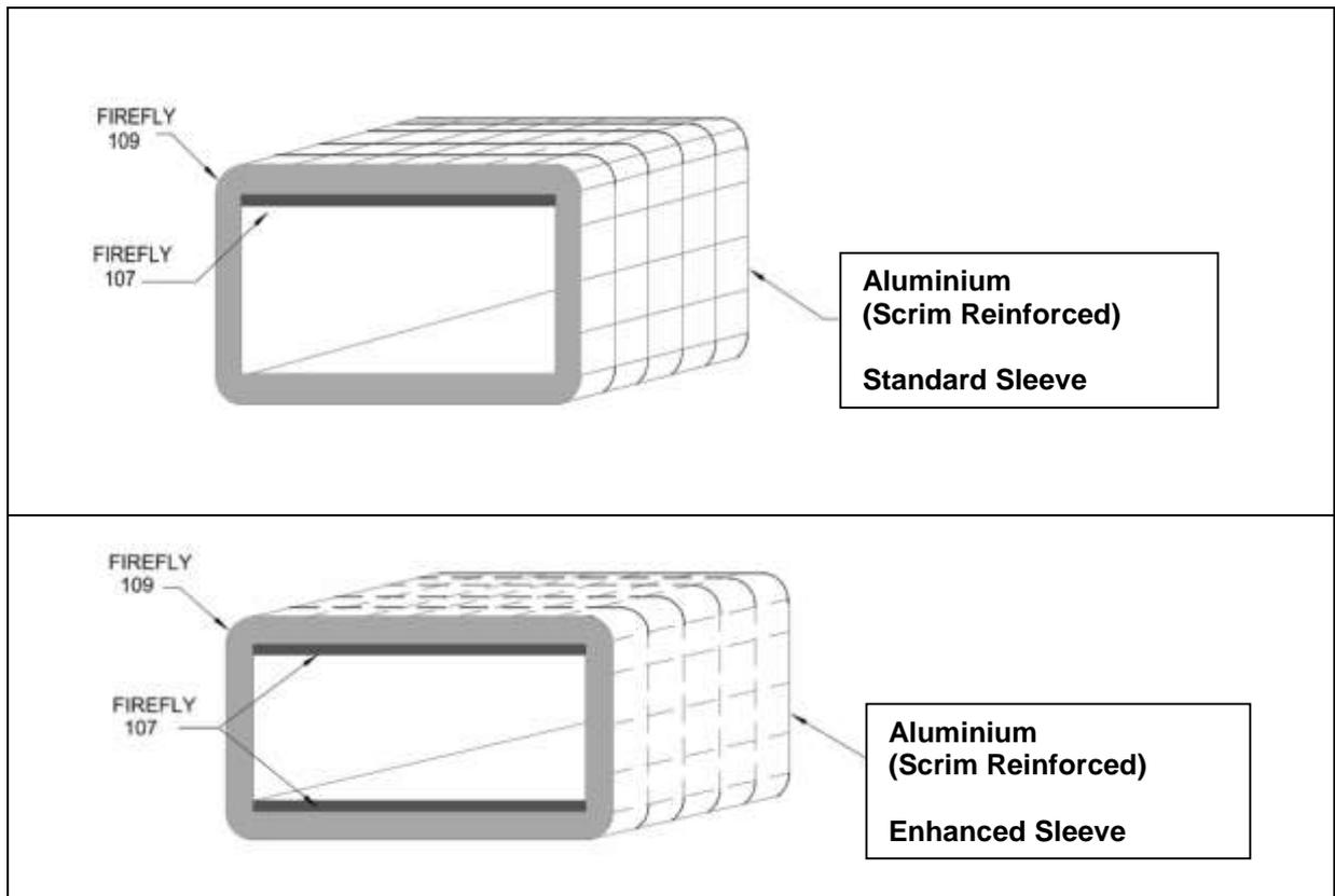
The Firefly 109+ LP Fire Sleeve – Rectangular is delivered in various sizes to fit particular duct sizes – see table below:
