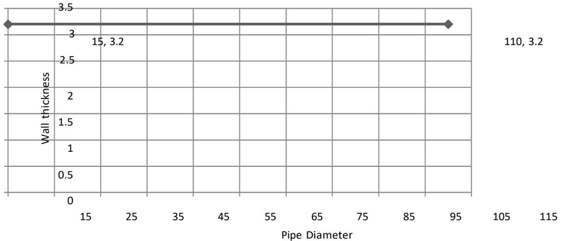
**B.4 Field of application for Tenmat Firefly 109 Fire Sleeve – Rectangular. For PVC-U rectangular ambient pressure extraction and ventilation ‘duct’ type pipes penetrating fire resistant walls for applications up to EI120:**
