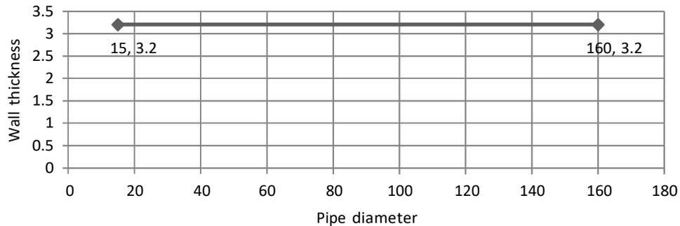
**B.7 Field of application for Tenmat Firefly 109 Fire Sleeve – Circular for PVC-U (according to EN 1329-1)\* and HDPE (according to EN 1519-1)\* pipes penetrating fire resistant floors for applications up to EI120:**
