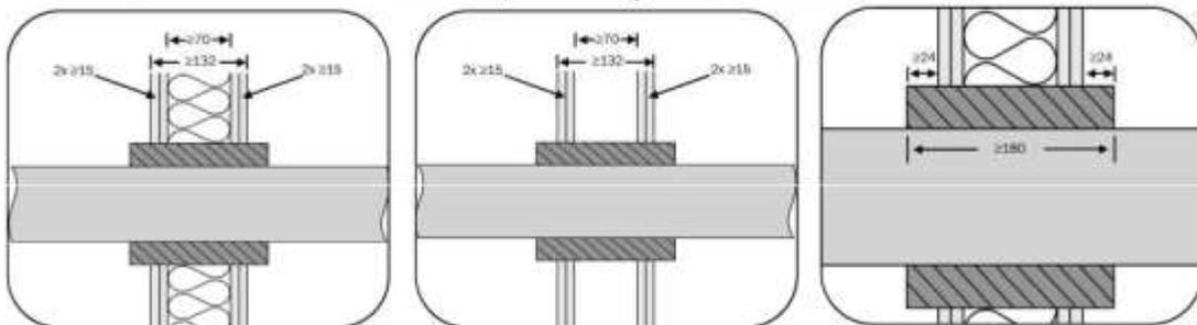
For timber stud partitions, seal must be  $\ge 100$ mm from studs with  $\ge 100$ mm of insulation (A1 or A2 to EN13501-1) between seal & stud.
