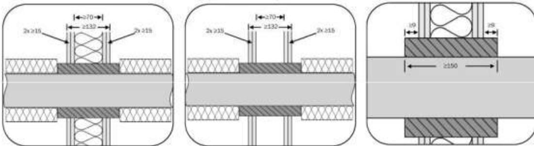
For timber stud partitions, seal must be  $\geq 100\text{mm}$  from studs with  $\geq 100\text{mm}$  of insulation (A1 or A2 to EN13501-1) between seal & stud.
