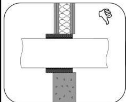
Rigid walls must comprise concrete, aerated concrete or masonry  $\geq 650\text{kg/m}^3$  (Wall Type A) or concrete, masonry  $\geq 1100\text{kg/m}^3$  (Wall Type B)
