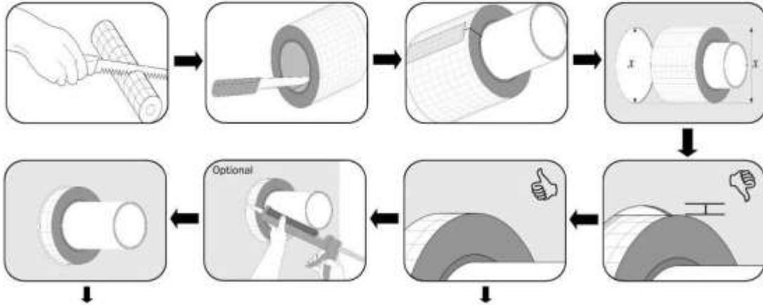
**Wall Penetrations - Plastic Pipes - Drywall Partition**
