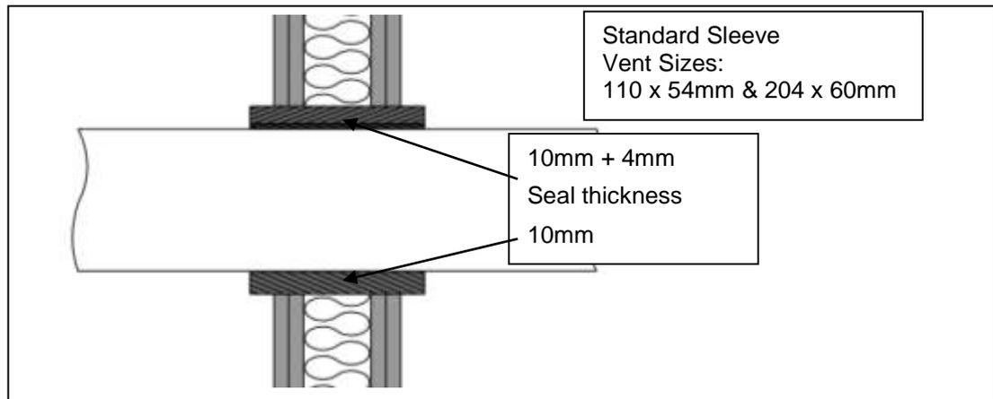
**D.6 Field of application for Tenmat Firefly 109+ LP Fire Sleeve – Rectangular (Enhanced Sleeve) for use with a 220mm wide x 90mm high PVC-U rectangular ambient pressure extraction and ventilation ‘duct’ type pipe penetrating fire resistant walls for applications up to EI120:**
