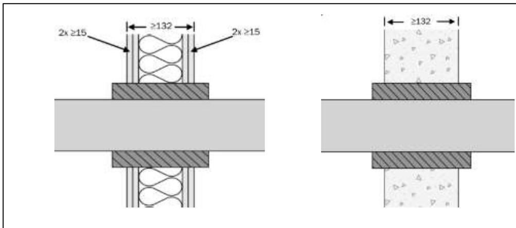
The seal must be a minimum of 280mm long with 74mm protruding each side
