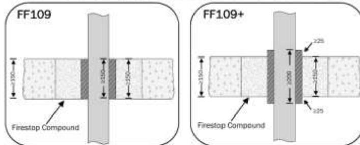
Rigid floors must comprise concrete  $\geq 2400\text{kg/m}^3$  (Floor Type A) or  $\geq 550\text{kg/m}^3$  (Floor Type B)
