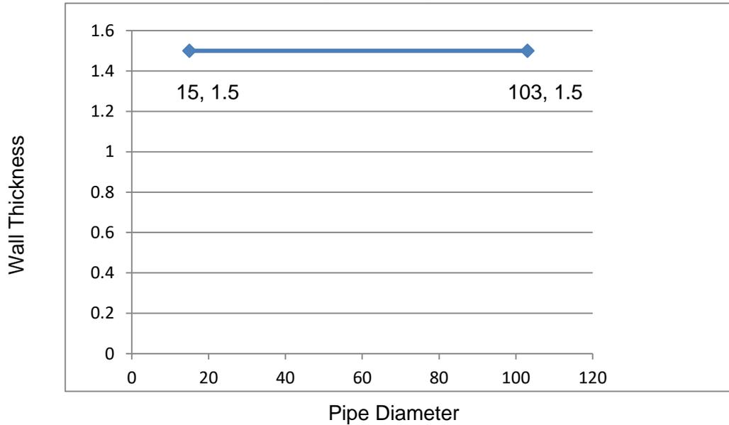
**D.2 Field of application for minimum 250mm long Tenmat Firefly 109+ LP Fire Sleeve – Circular (Standard Sleeve) for PVC-U circular ambient pressure extraction and ventilation 'duct' type pipes penetrating minimum 100mm thick fire resistant walls for applications up to EI120:**
