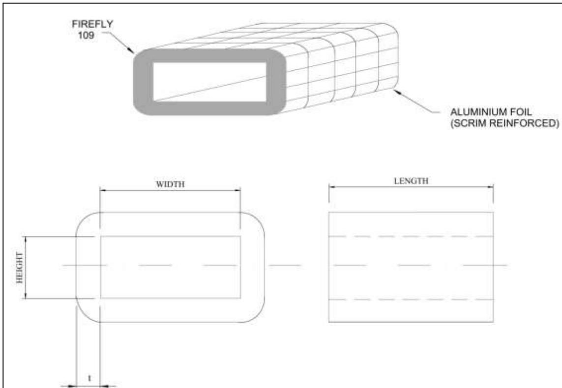
The Firefly 109 and 109+ Fire Sleeve – Rectangular is available as single sleeve up to 500mm long which can be cut down to suit the intended application. It must be a minimum of 180mm long or longer if the supporting construction is thicker. The Firefly 109 and 109+ is delivered in various sizes to fit particular duct sizes – see table below:
