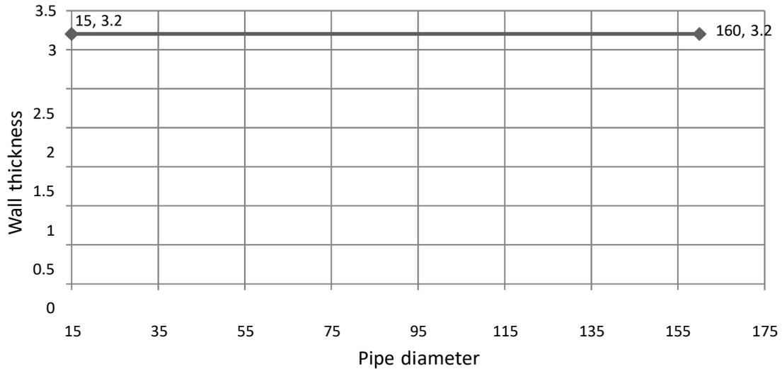
**C.1.3 The line graphs below show the coverage of the allowable HDPE (according to EN 1519-1)\* pipe diameters and wall thickness for applications up to EI120:** (any pipe size variation along the line is covered)
