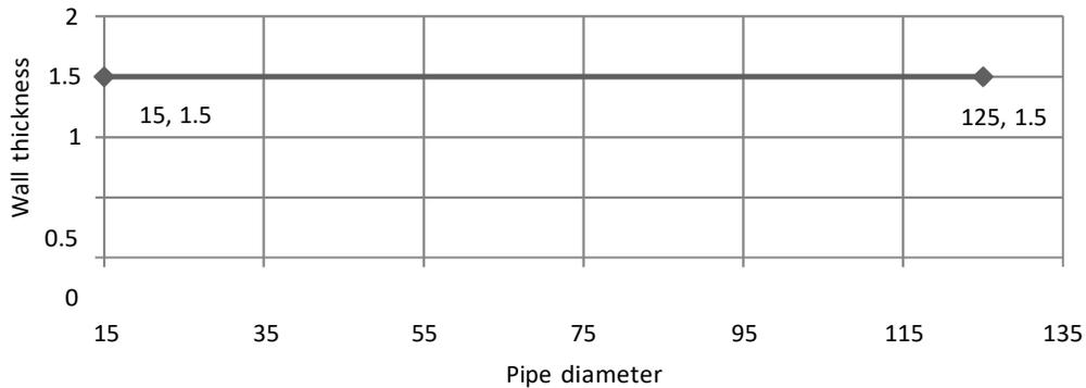
**C.4 Field of application for minimum 150mm long Tenmat Firefly 109+ Fire Sleeve – Circular for PVC-U (according to EN 1329-1)\* pipes penetrating fire resistant masonry walls only for applications up to EI240**
