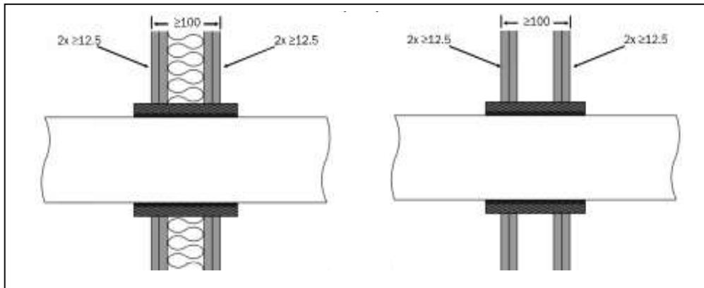
The seal must be a minimum of 250mm long with 75mm protruding each side
