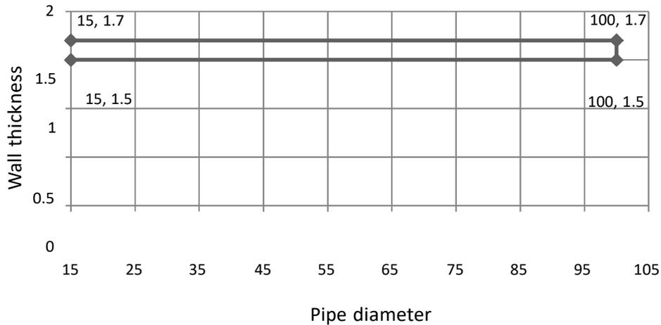
**C.3** Field of application for minimum 280mm long Tenmat Firefly 109+ Fire Sleeve – Circular for PVC-U circular ambient pressure extraction and ventilation 'duct' type pipes penetrating fire resistant walls for applications up to EI120:
