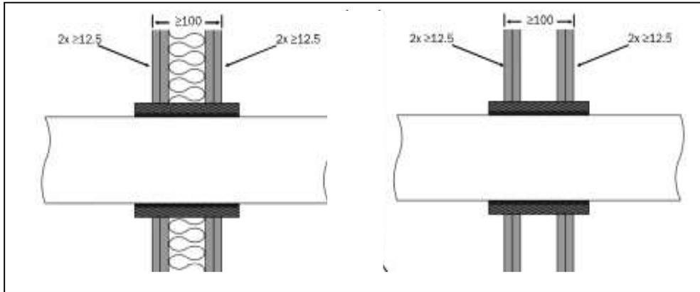
The seal must be a minimum of 150mm long with 25mm protruding each side
