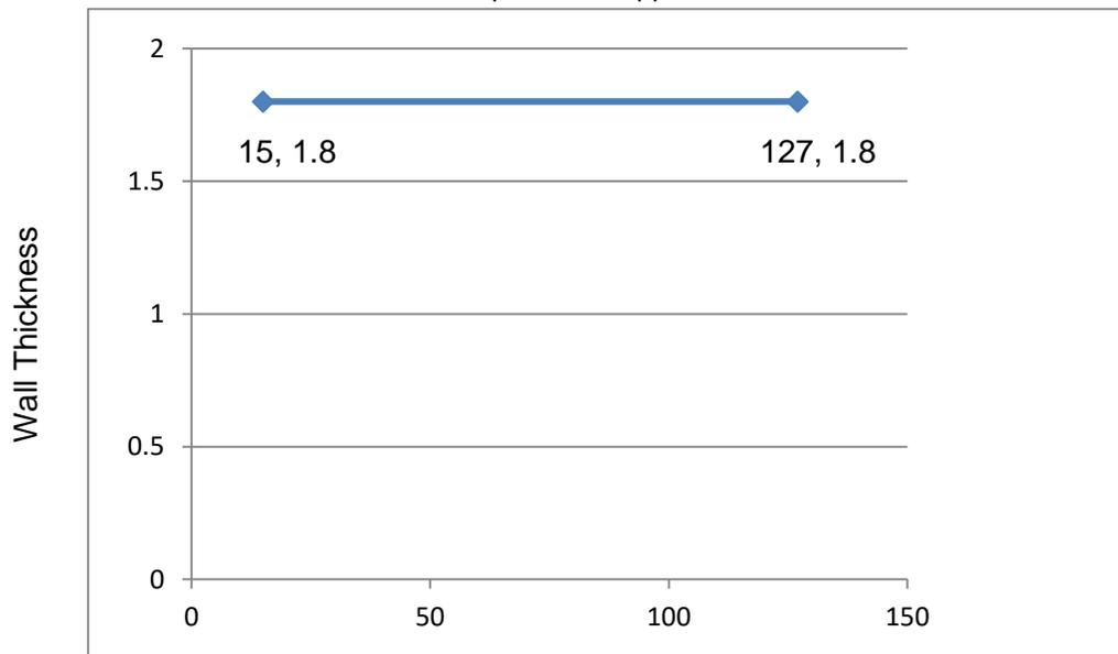
**D.3 Field of application for mini Pipe Diameter Fenmat Firefly 109+ LP Fire Sleeve – Circular (Enhanced Sleeve) for PVC-U circular ambient pressure extraction and ventilation ‘duct’ type pipes penetrating fire resistant walls for applications up to EI120:**
