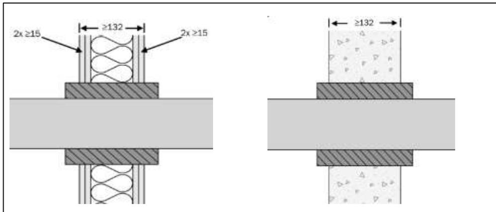
The seal must be a minimum of 150mm long with 9mm protruding each side of the wall
