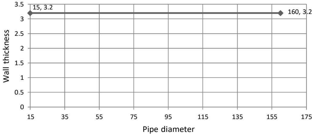
**C.7.2 The line graph below shows the coverage of the allowable HDPE (according to EN 1519-1)\* pipe diameters and wall thickness for applications up to EI120: (any pipe size variation along and between the lines is covered)**
