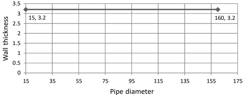
**C.6.2** The line graph below shows the coverage of the allowable HDPE (according to EN 1519-1)\* pipe diameters and wall thickness for applications up to EI120: (any pipe size variation along the line is covered)
