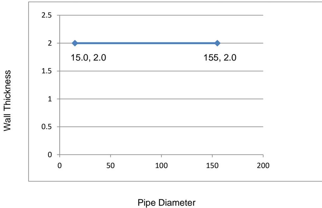
**D.4 Field of application for Tenmat Firefly 109+ LP Fire Sleeve – Rectangular (Standard Sleeve) for use with a 204mm wide x 60mm high PVC-U rectangular ambient pressure extraction and ventilation ‘duct’ type pipe penetrating fire resistant walls for applications up to EI120:**
