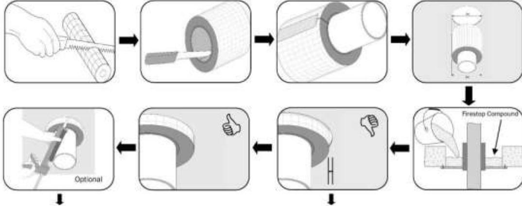
**Floor Penetrations - Plastic Pipes - Solid Floor**
