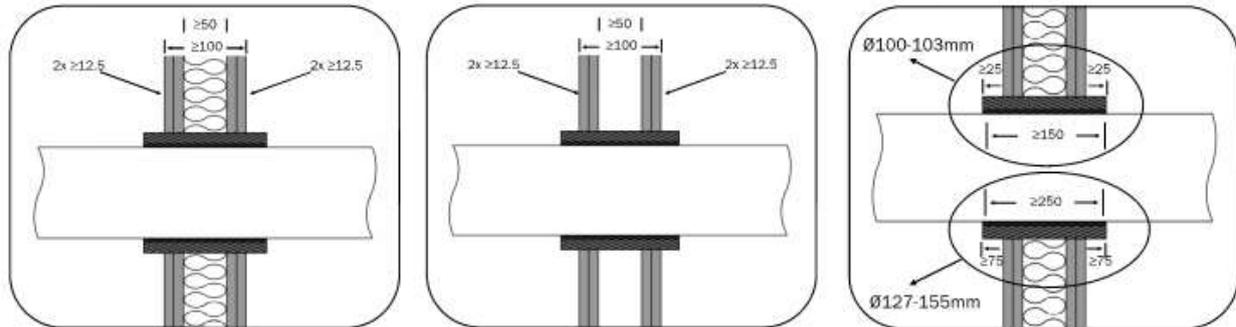
For timber stud partitions, seal must be  $\geq 100\text{mm}$  from studs with  $\geq 100\text{mm}$  of insulation (A1 or A2 to EN13501-1) between seal & stud.
