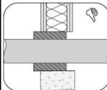
Rigid walls must comprise concrete, aerated concrete or masonry  $\geq 650\text{kg/m}^3$  (Wall Type A) or concrete, masonry  $\geq 1100\text{kg/m}^3$  (Wall Type B)
