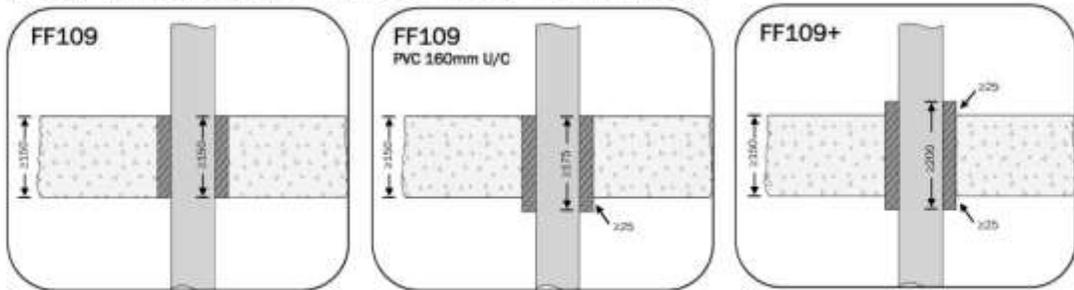
Rigid floors must comprise concrete  $\geq 2400\text{kg/m}^3$  (Floor Type A) or  $\geq 550\text{kg/m}^3$  (Floor Type B). For further details check the ETA
