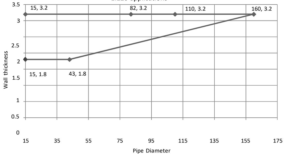
**B.2.2 The line graphs below show the coverage of the allowable HDPE (according to EN 1519-1)\* pipe diameters and wall thickness for applications up to EI120: (any pipe size variation along the lines and the area between the lines is covered)**
