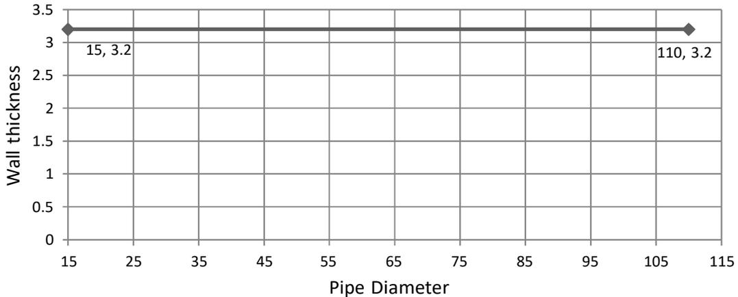
**B.8.3** The line graph below shows the coverage of the allowable HDPE (according to EN 1519-1)\* pipe diameters and wall thickness for applications up to EI120: (any pipe size variation along the line is covered)
