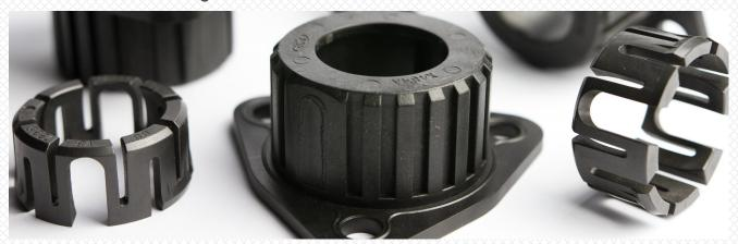
TENMAT RAILKO PV80 is based on an acetal copolymer with mineral oil encapsulated in micro pockets throughout the matrix. This structure ensures self lubrication for life, combined with good dimensional stability, very low swell in water, and good creep resistance. PV80 has
