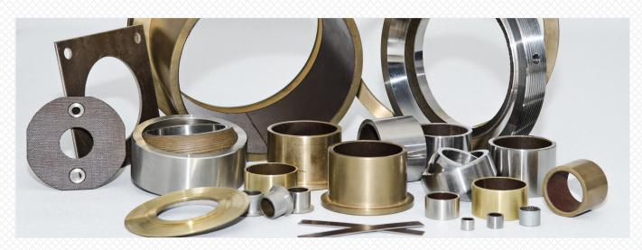
**TENMAT** FEROGLIDE T401 bearing material is a self-lubricating, resin impregnated hybrid cloth with PTFE fibres on the wear surface, bonded onto 316 stainless steel or Inconel 625 with special high temperature adhesive.
