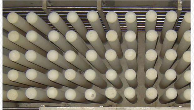
**TENMAT** Hot Gas Filter Elements are industry leaders and have shown to be significantly stronger than competitive materials, especially when operating at high temperatures. **TENMAT** Hot Gas Filter elements effectively filter both micron and sub micron particles.
