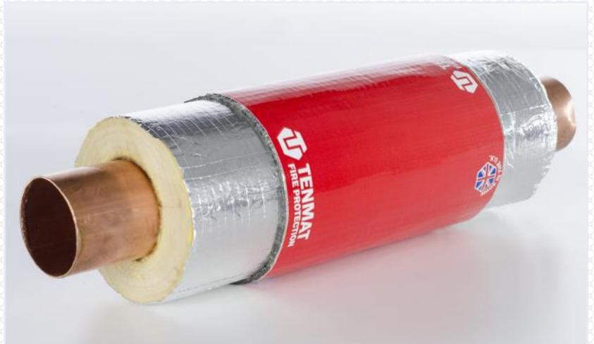
The **TENMAT FIREFLY** OverSleeve is a universal, one-product-fits-all solution for the firestopping of insulated metal pipes. The thin and flexible intumescent is quickly and simply wrapped directly on top of pipe insulation without the need to cut back, ensuring that thermal and vapour seal performance is maintained. The red branded foil can be easily checked and identified on site to confirm that firestopping is in place.
