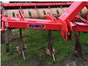
“This subsoiler was fitted with these scrapers and has since completed over 3000 acres of abrasive sand land.
