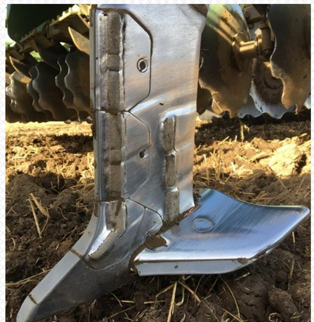
The point below would typically complete 250 acres on a 5metre cultivator before wearing out. After applying Ferobide behind the tungsten in 3 rows this point has already completed 650 acres.
