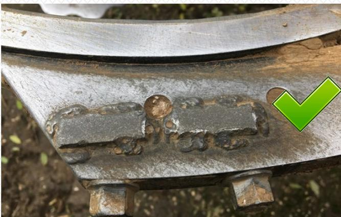
Ferobide is welded quickly and cost effectively directly to the area of wear on the side. Ferobide is a proven solution, as shown on the left.
