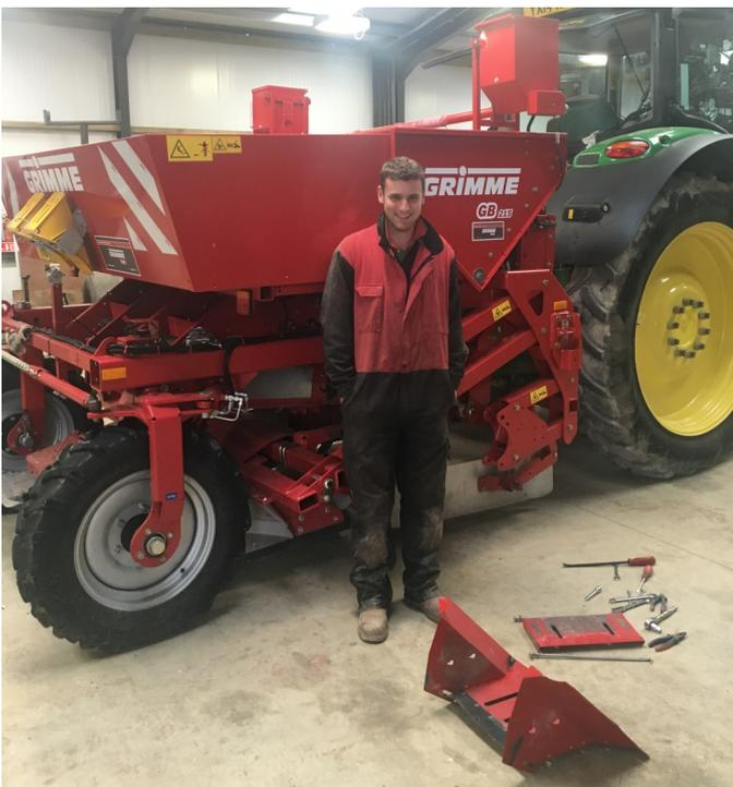
“We welded Ferobide onto the openers and it looks they will last 5 times as long as standard.
