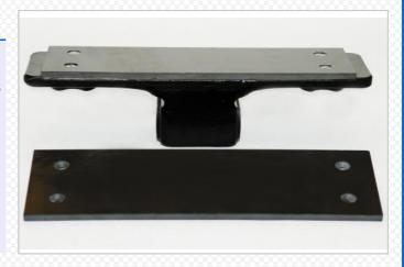
**TENMAT**'s RAILKO NF21 fully UIC approved Side Bearer Liners are installed onto the sides of the freight bogie to provide support to the car body. RAILKO plates are used to help safely manoeuvre the bogie and car body around curves on the track.
