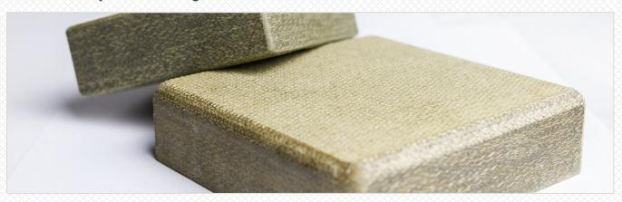
**TENMAT** FEROFORM F363 is a cured phenolic resin matrix reinforced with a woven glass/aramid fibre cloth with a friction modifier evenly dispersed throughout the matrix.
