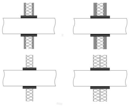
Single double layer or plasterboard. Approved with or without cavity insulation for all duct sizes listed
