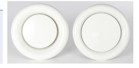
The **TENMAT** FIREFLY Fire Rated Ceiling Air Valves are a unique and cost effective fire rated solution where recessed ceiling air valves are to be installed in fire rated ceilings. In a fire situation, the integral intumescent material rapidly expands to seal off the air valve and reinstate the fire resistance rating of the ceiling. This limits the risk of fire and heat spread throughout the building. The **TENMAT** Ceiling Air Valves are available in all sizes for both Extract and Supply.
