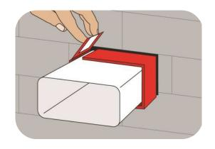
The Fire Wraps are easily wrapped around the vent duct due to the four segment design and slid into the wall construction. In a fire situation the high expansion intumescent material will rapidly expand to effectively seal off the vent duct to prevent the passage of fire and hot gasses.
